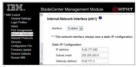
Figure 6-3 Management Module Internal Network Interface window
